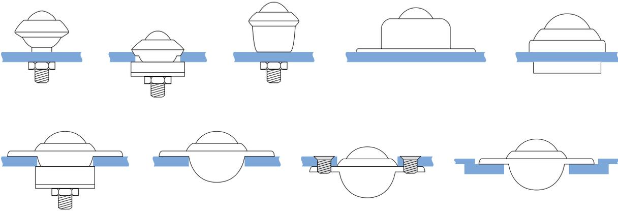
There are various methods of fixing ball units. A wide range of fittings enable them to be used with various different materials. Fixing clips are available for most designs.
