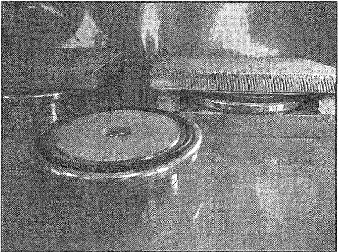
Sliding bearings for high temperatur varying
